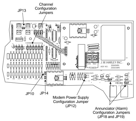
Figure 3-3: I/O Board Configuration Jumper Locations
